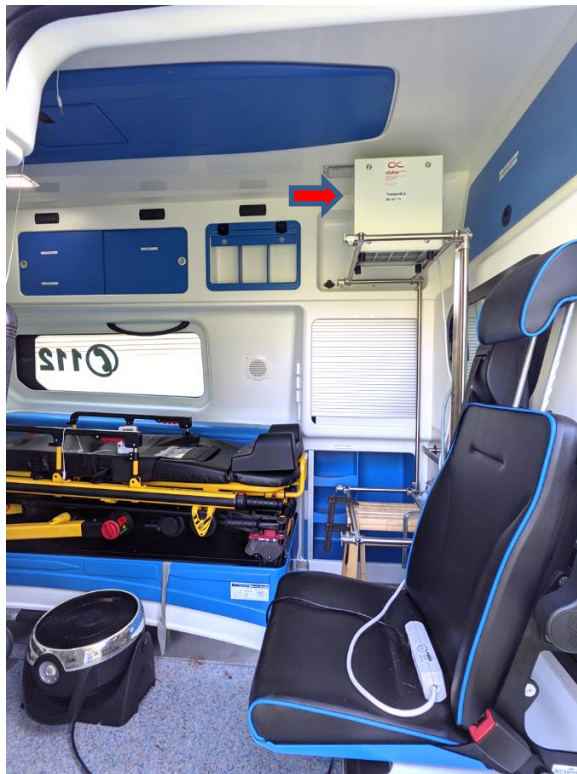
Figure 2 Experimental setup in the emergency car. The ionizer is located on the stainless steel frame (top right).
